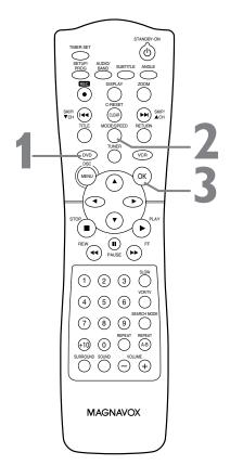
Press TUNER to select Tuner mode. The red TUNER light will appear on the front of the System. The current radio frequency (station number) will appear on the display panel.
